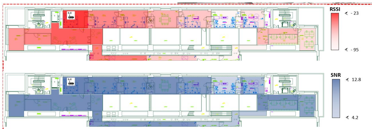
Figure 4: signal coverage simulation at the 3rd floor of the A2 building of the NOI Techpark.
